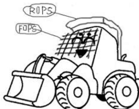
Soil piled on the ground or beside canals is soft and sloppy. The weight or vibration of the machine may collapse the soft soil that cause machine turnover.
