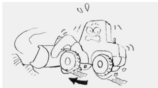
Do not let the machine close to the edge of a cliff or its hanging parts and deep pit.
