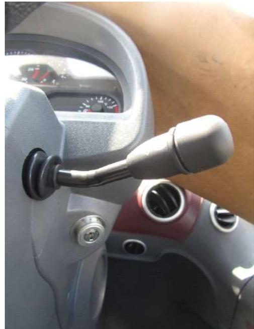
1. **OFF**-- When the starter switch key stays at this position, the power supply to loader will be cut off. The loader is off, i.e. automatic stop.
