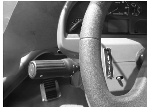
**NOTE: When carrying out gear-shifting operation, release the accelerator pedal firstly and then operate the gear-shifting lever for realizing the gear shifting, so as to protect the gear-shifting clutch.**
