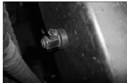
6. Re-fill soft water into the engine and add proper amount of special cleaning agent with the same filling method as that of the coolant.
