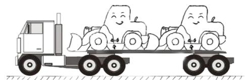
Check whether its loading capacity can support the weight of the machine when passing through a bridge or a structure.
