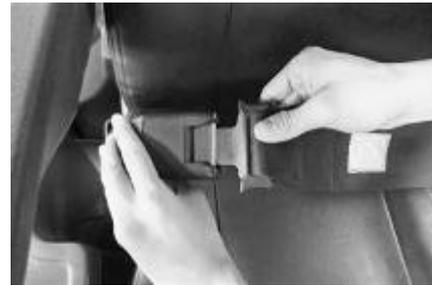
Press the red button near the anchorage, the buckle will spring out.
