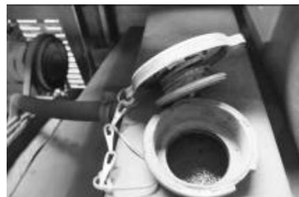
1. Slowly uncap the pressure cap at the upper section of the heat radiator, and gradually release the pressure.
