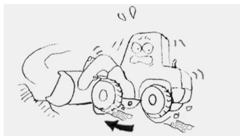
Avoid operating on the cliff edge, suspended material or deep pit, if the ground collapsed, the machine crashed or upset, which may cause serious casualties. Especially after raining, do blasting operations or after earthquake, the soil is very soft and sloppy and prone to cause danger.
