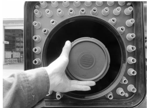
5. Blow away the dust on the filter paper of coarse filter with compressed air free of oil mist, water (pressure less than 300KPa). (After coarse filter is cleaned five times, it is needed to replace air fine filter and cleaned fine filter shall not be used again.)
