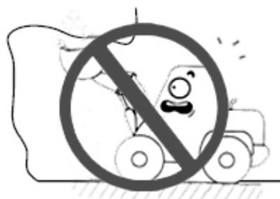
Please install head protection devices for operation on dangerous areas where there are falling stones.
