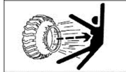
Equipments and staff are needed to avoid over-inflation. Leakage or rim damage is due to the incorrect or improper use of inflatable equipment. When inflating tire, you should stand on the side and use automatic working clamp.
