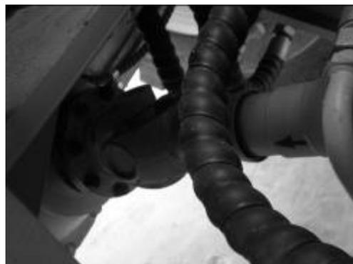
If it is suspected that the gearbox fails, just dismantle the front/rear transmission shafts and then get the loader towed.
