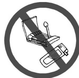
Do not use mobile phone when operating the loader, because distraction may cause accidents.
