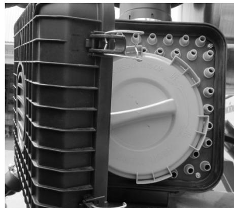
2. Unscrew the filter cover in arrow direction.
