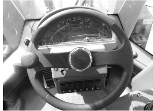
The loader is equipped with the articulated-type fully-hydraulic coaxial-flow-amplifying powered steering gear, and the turning angle of the steering wheel is not equal to the turning angle of the loader. When the steering wheel is turned continuously, the turning angle of the loader will increase until the intended angle is obtained. The turning speed of the loader will increase as the turning speed of the steering wheel increases.
