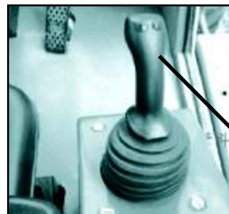
Palanca Control Cuchara
